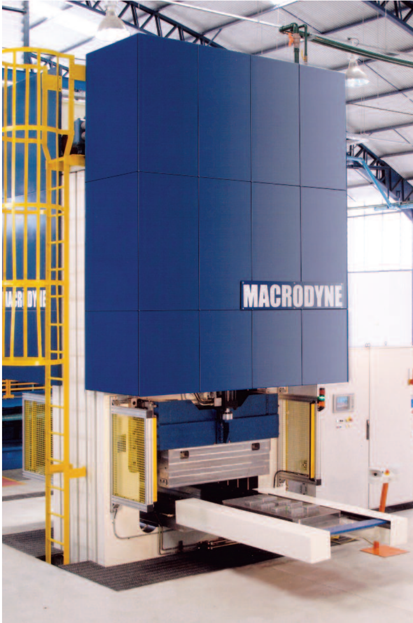
7700 ton elastoforming press with shuttle table
