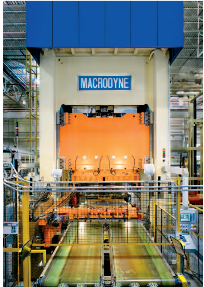
1200/4 x 200 ton single acting deep draw press with hydraulic cushion
