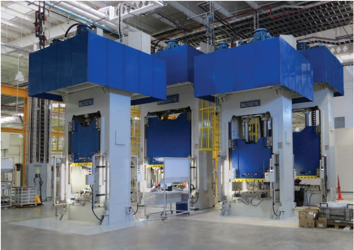
Three (3) 200 ton metalforming presses with two (2) 220/100 ton single-acting draw presses with hydraulic cushions
