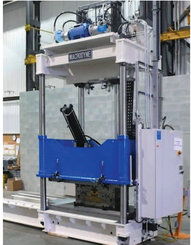
50 ton die spotting press with 90 degree tilting platen and sliding table
