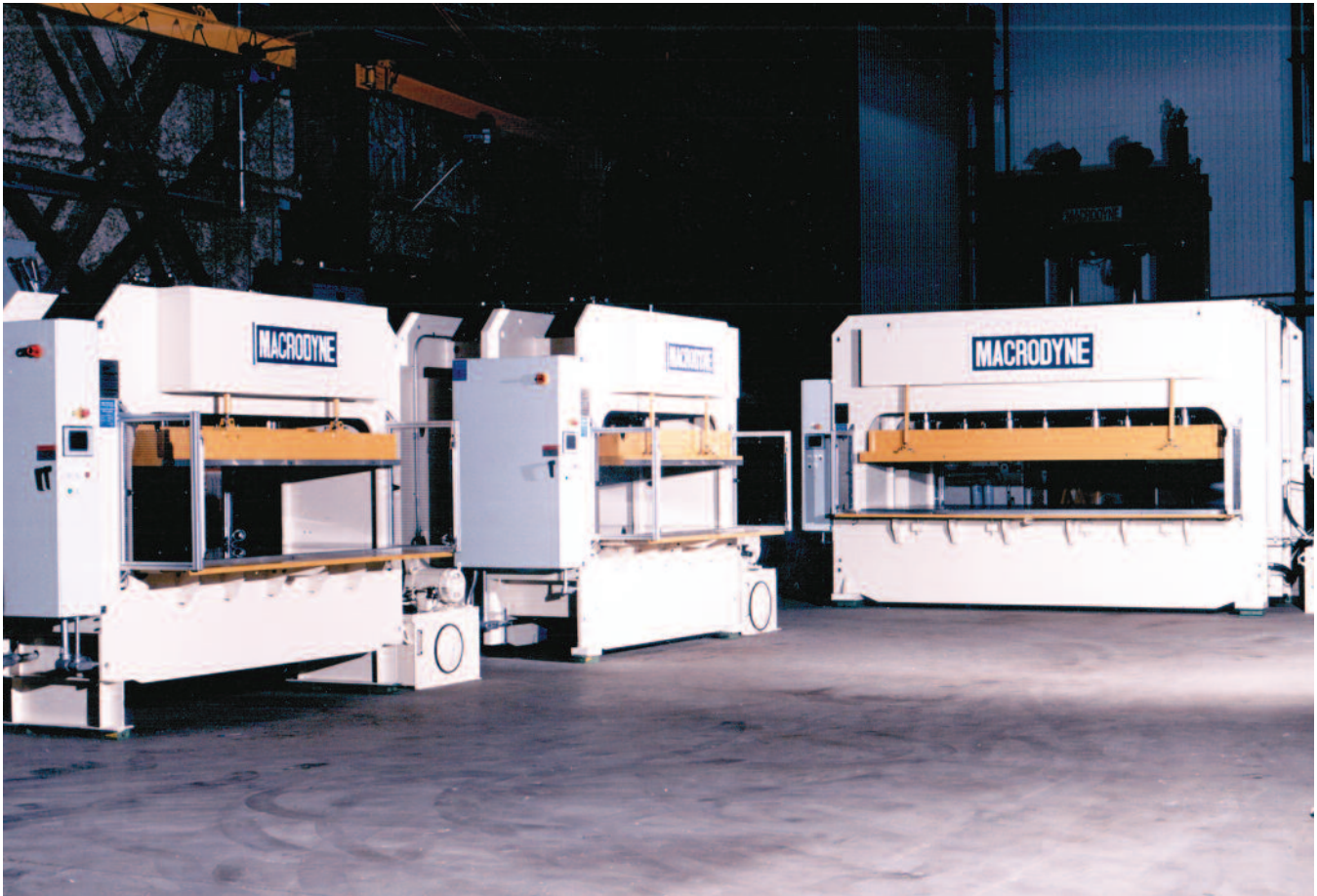
480 ton, 240 ton, and 40 ton low pressure bonding presses
