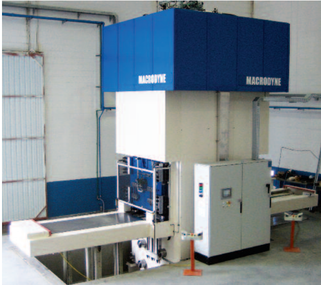
11,000 ton press with dual shuttle tables
