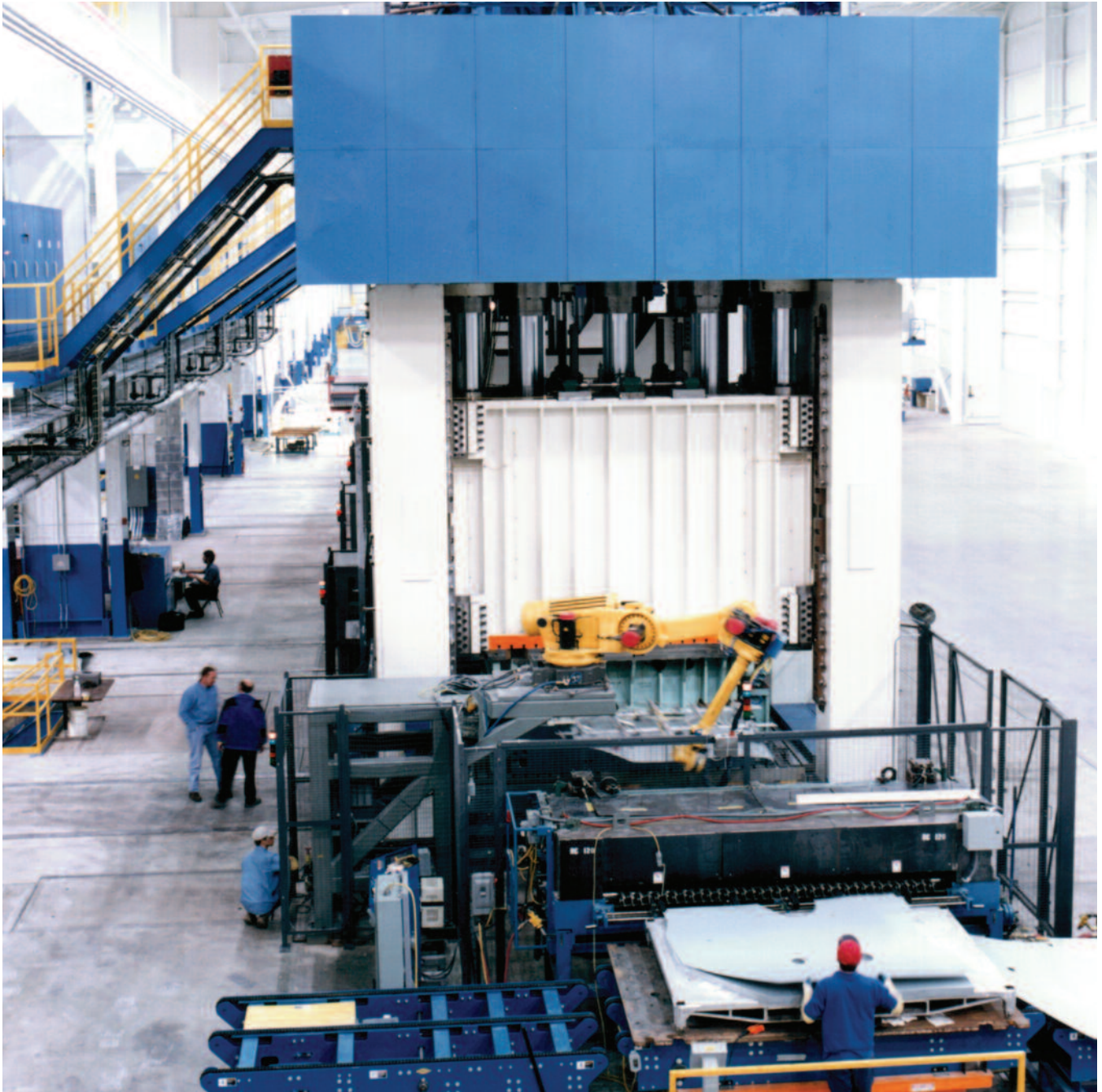
1600/900/500 ton double-acting draw press with hydraulic cushion
