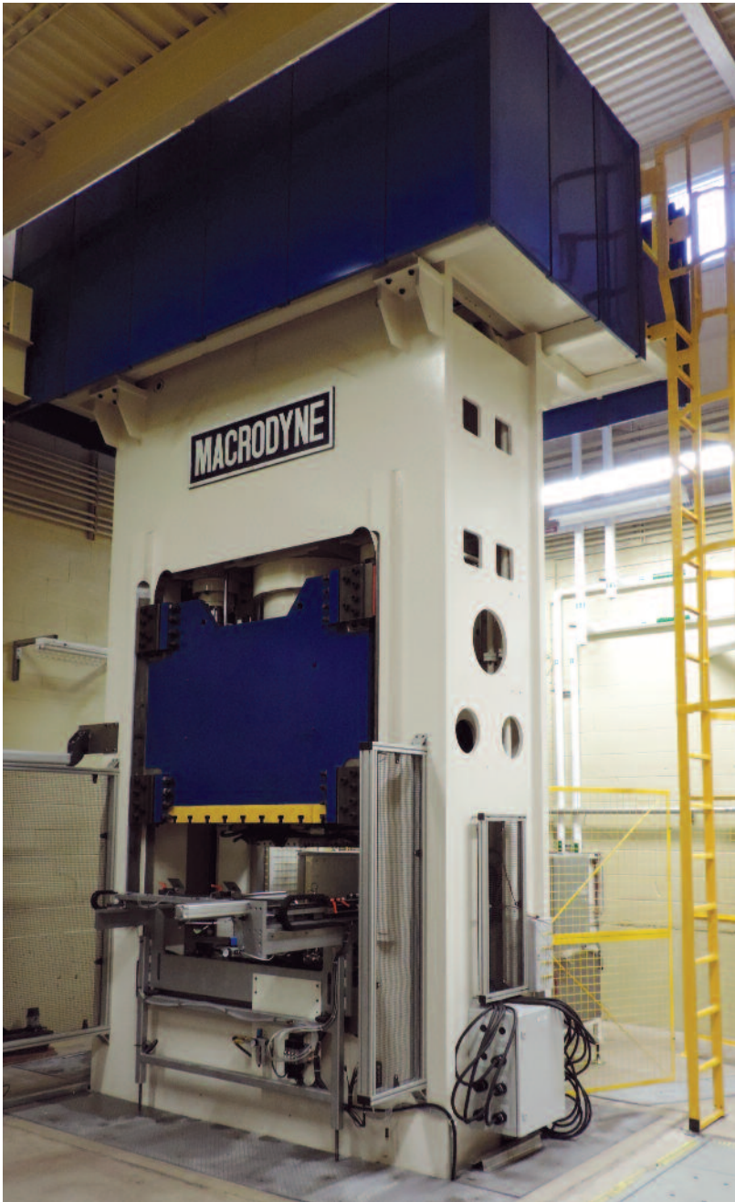
600/300/150 ton double-acting R&D press with hydraulic cushion
