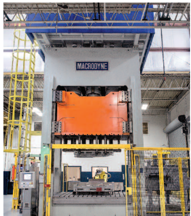
660/220 ton dual capability hot stamping/deep draw press
