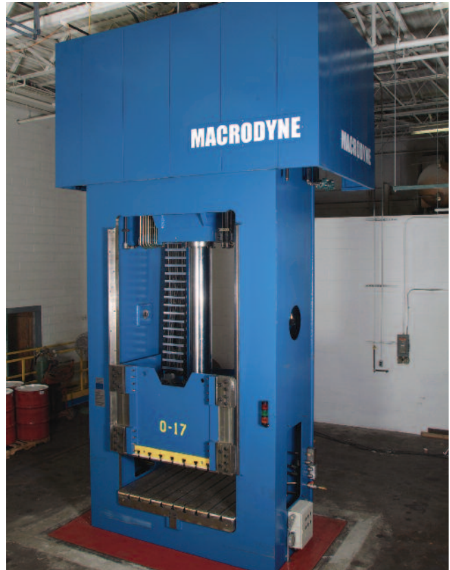
300 ton SMC compression molding presses
