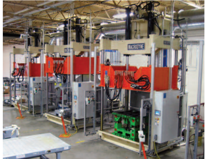
Four (4) 50 ton trim presses
