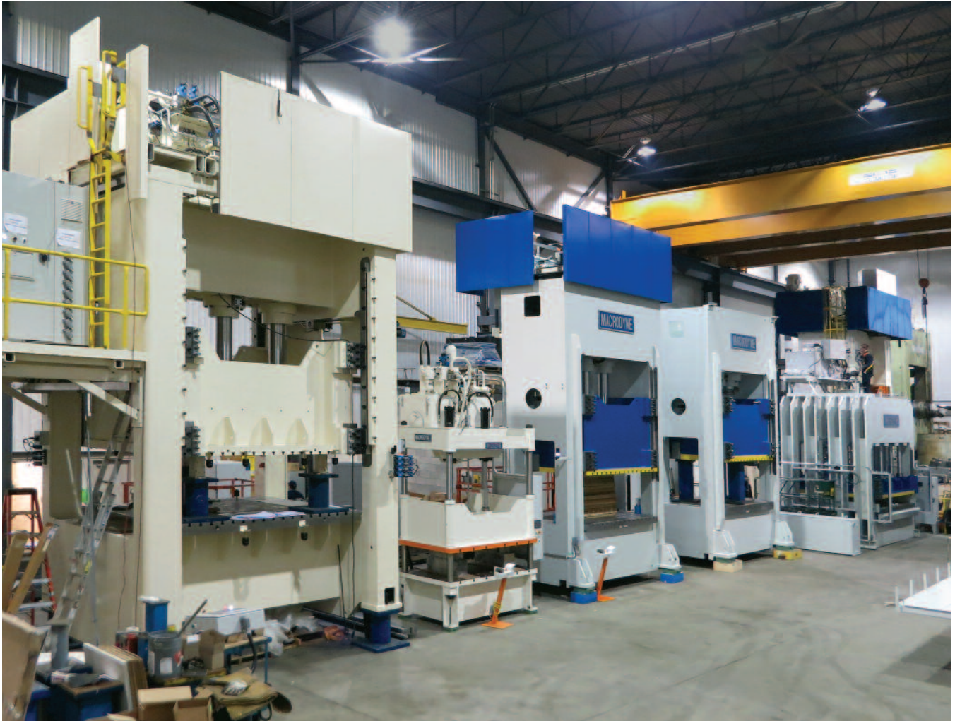
Variety of presses with different frame styles shown during assembly in our factory
