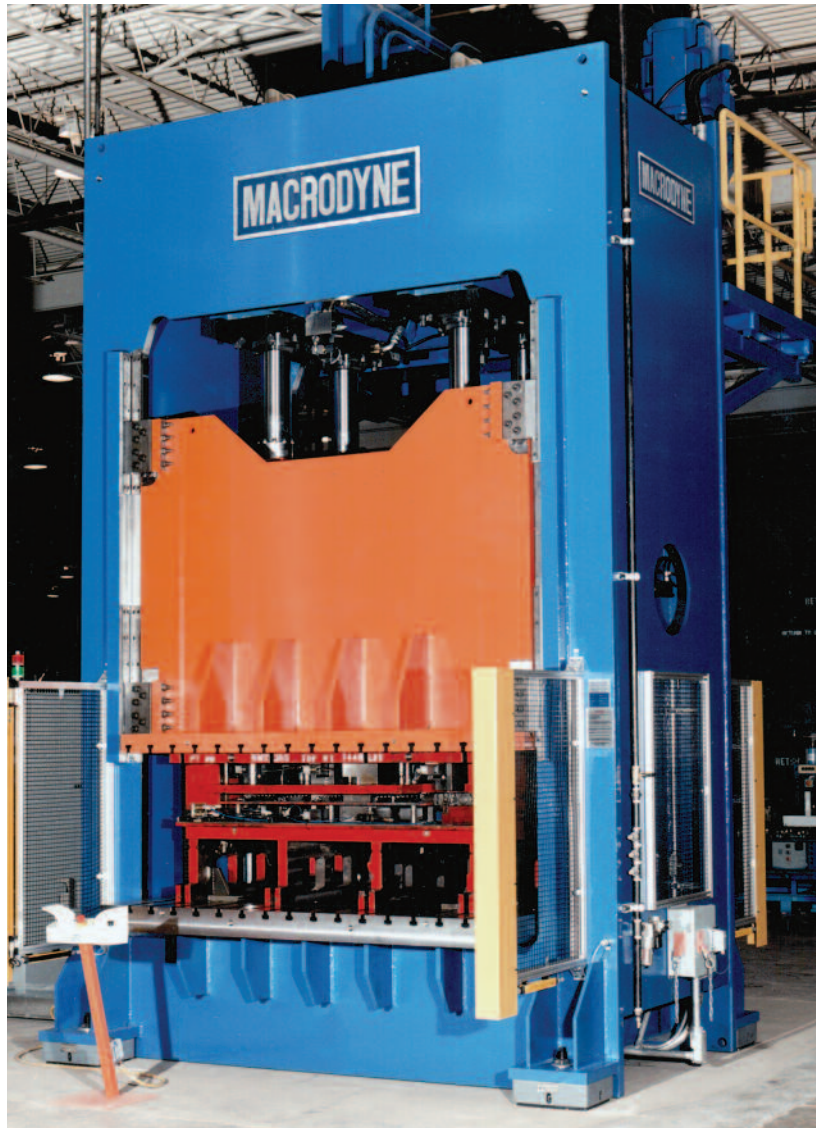
400 ton metalforming press featuring low headroom design
