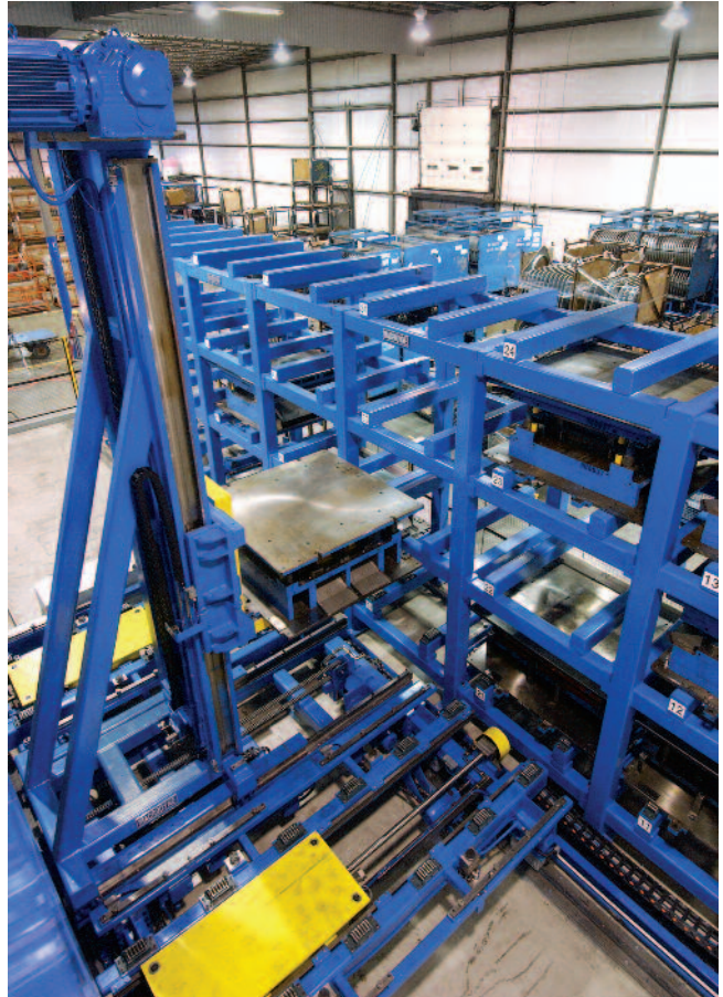
Die elevator with twin die load/unload devices
