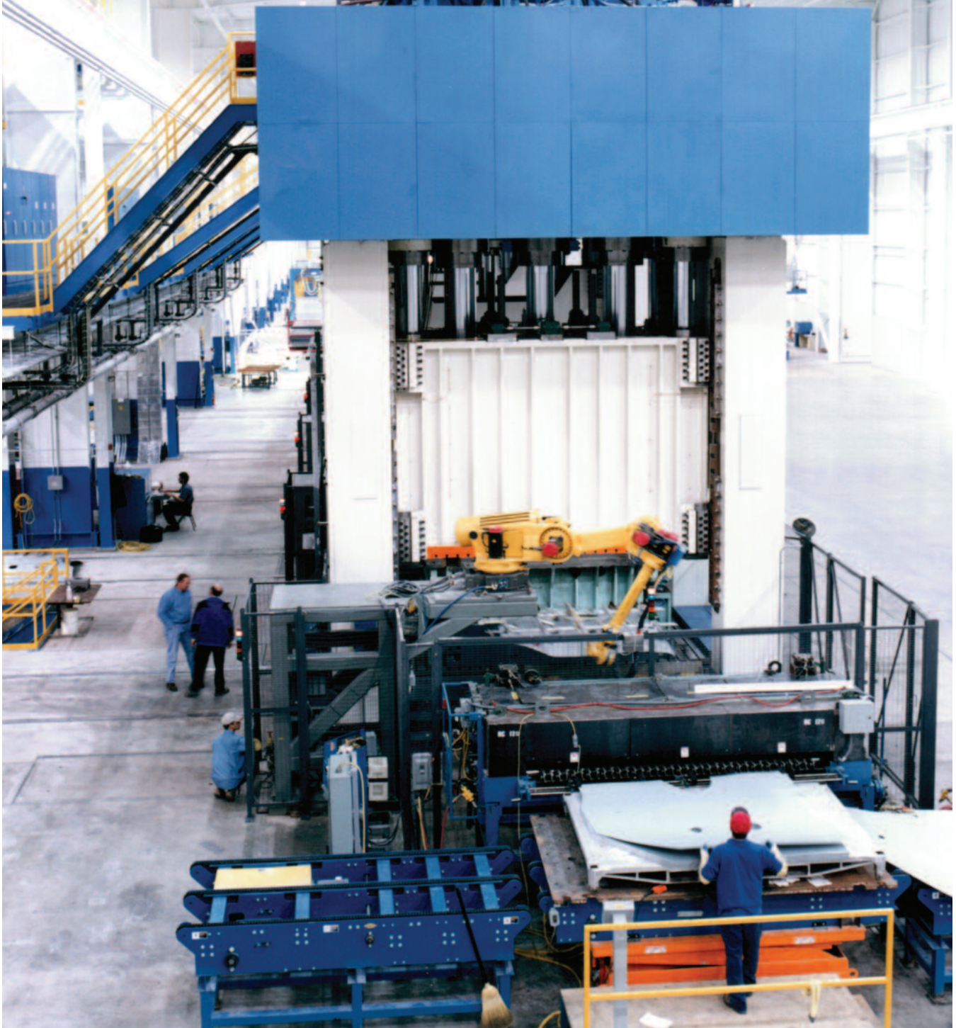
1600/900/500 ton double-acting deep draw press with hydraulic cushion and two (2) 180" x 96" rolling bolsters
