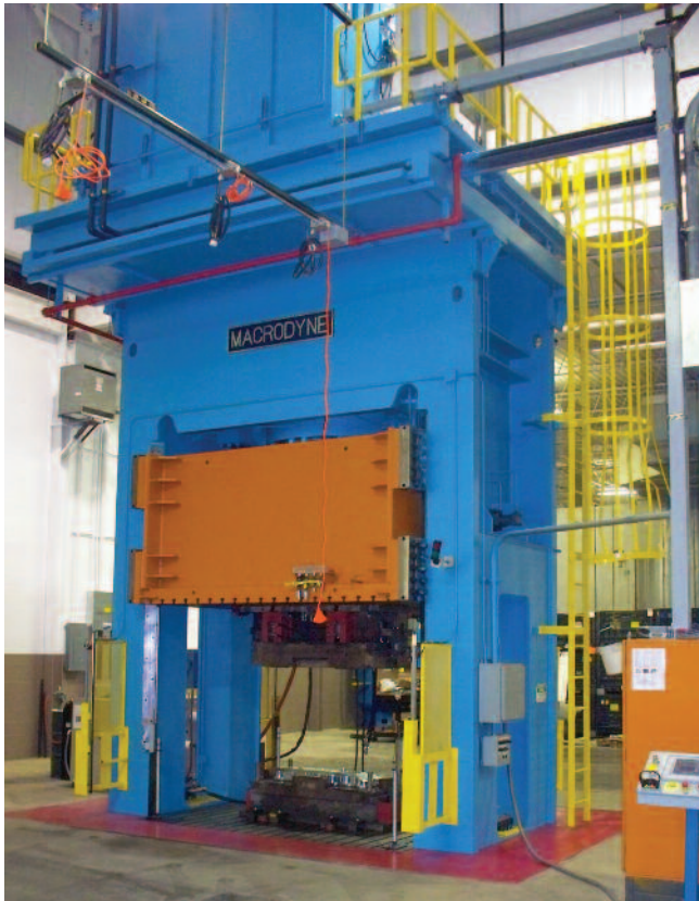
2000 ton SMC compression molding press
