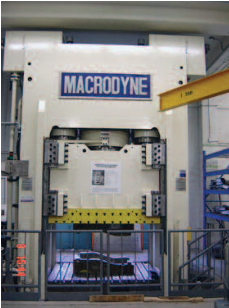
900/600/300 ton double-acting R&D press with multi-point blank holder and cushion
