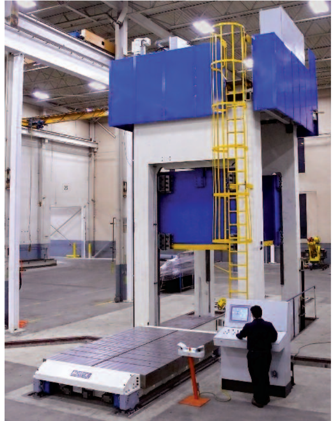
1000 ton press with two (2) side to side rolling bolsters
