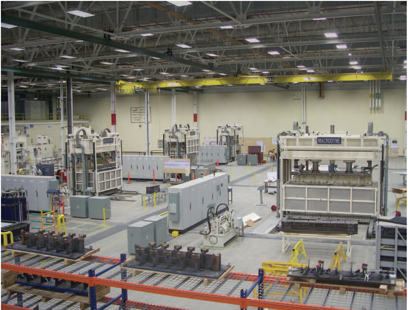
One (1) 700 ton & three (3) 600 ton super plastic forming presses
