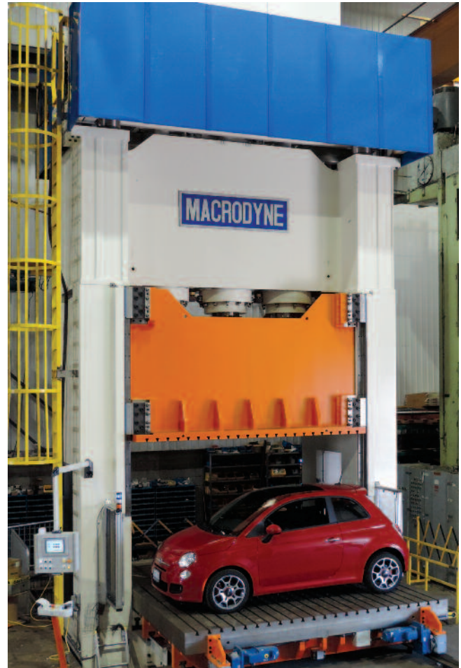
2000 ton single-acting draw press with hydraulic cushion & rolling bolster
