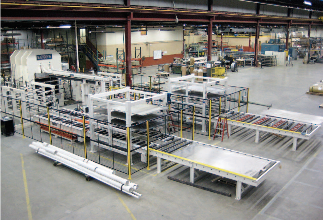
1500 ton, 4 daylight, heated platen press with automated loading/unloading systems
