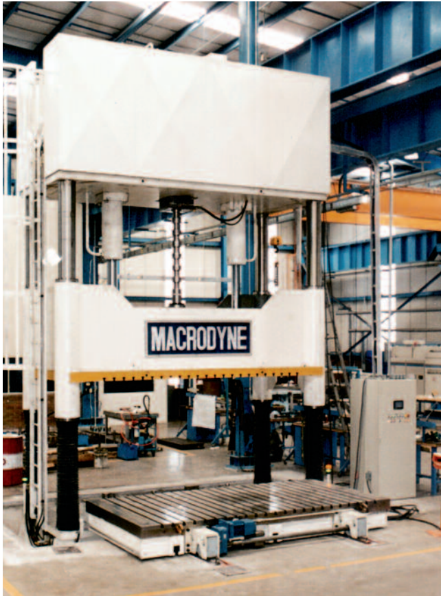
250 ton die spotting press with rolling bolster
