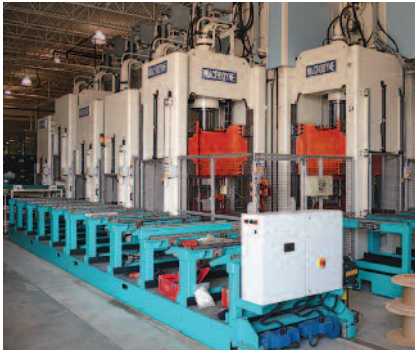
Hydraulic press line for automotive heat shields
