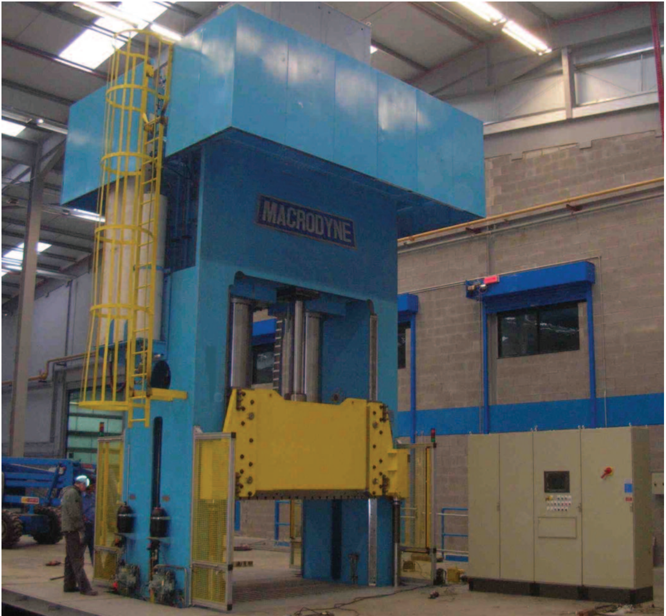
1600 ton SMC compression molding press
