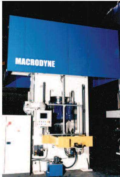
500/4x50 ton tube hydroforming press
