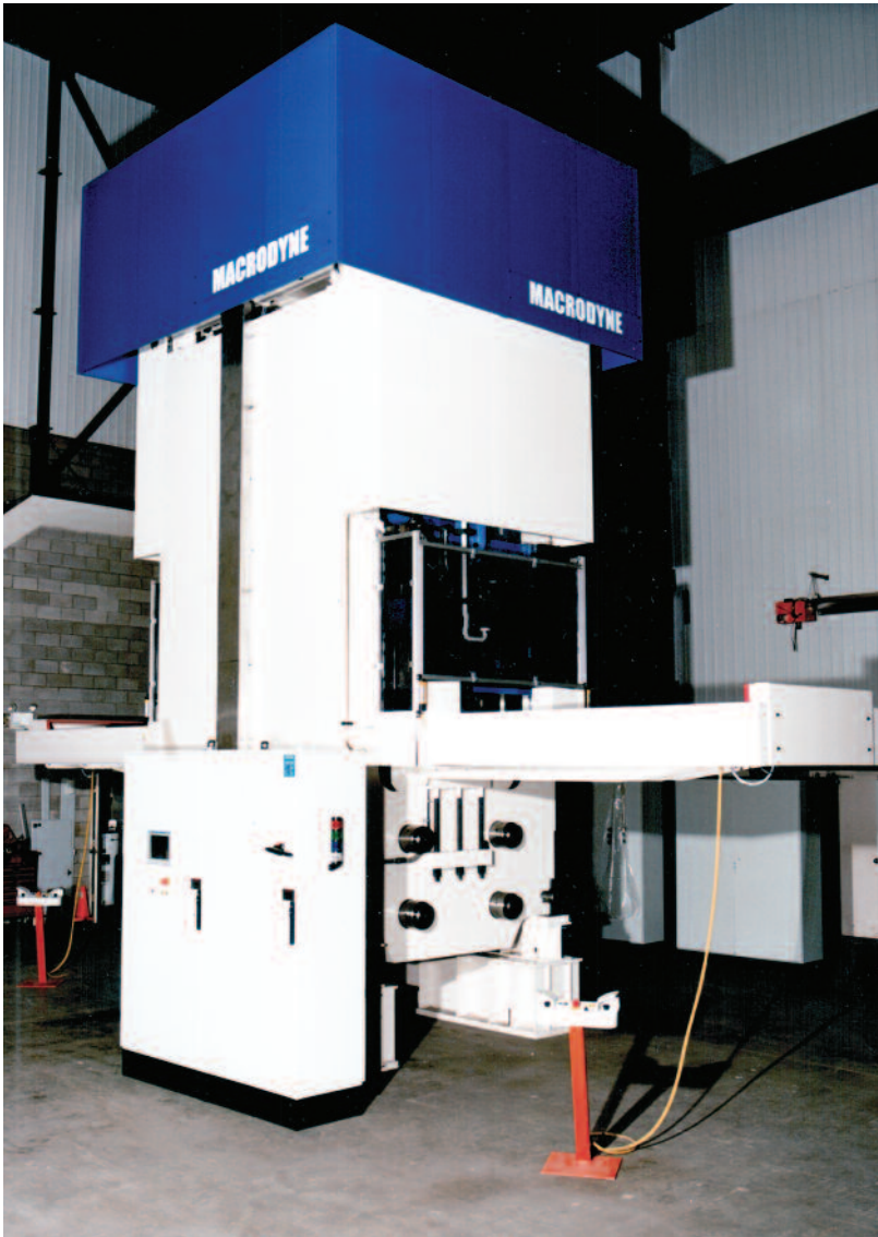
11,000 ton elastoforming press with dual shuttle tables
