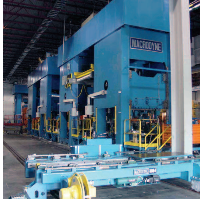
Die storage & retrieval system serving four (4) Macrodyne 500 ton presses and one (1) Macrodyne 2500 ton hydroforming press
