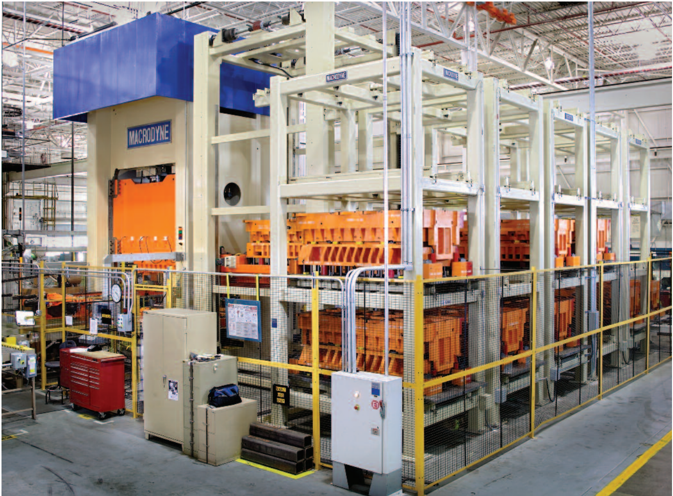
1200/4x200 ton single acting with cushion draw press served by a Macrodyne die storage & retrieval system
