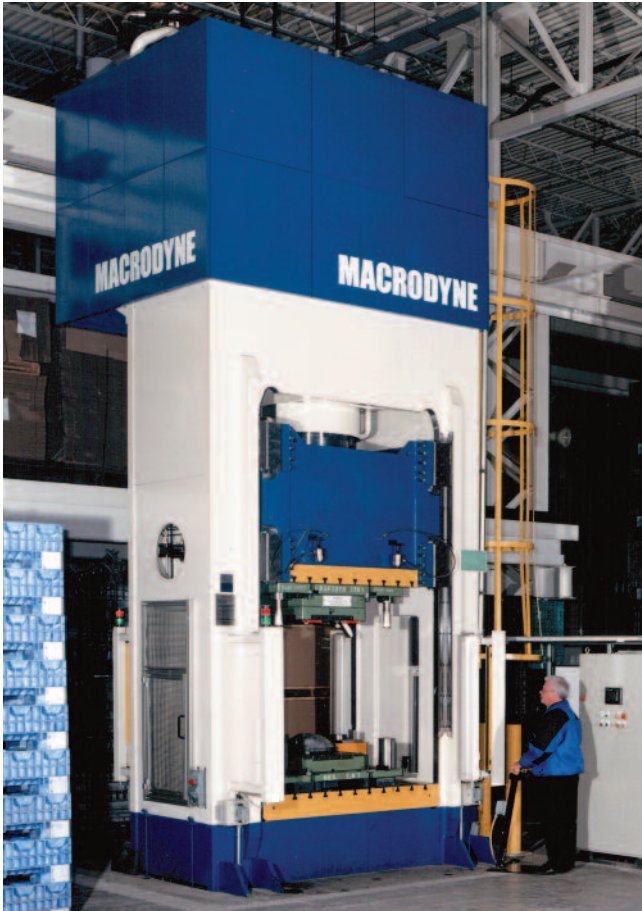
660 ton metalforming press with monolithic frame design
