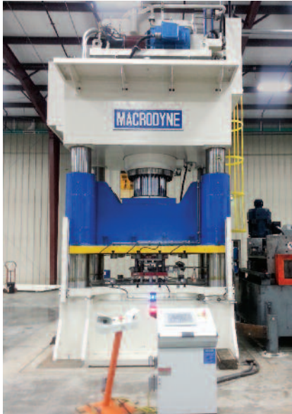
Rebuilt 1375 ton metalforming press
