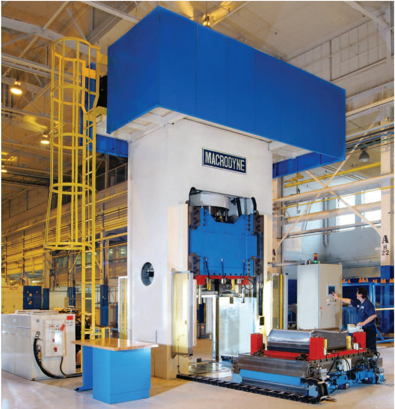
1100/200 ton single-acting deep draw press with hydraulic cushion and rolling bolster
