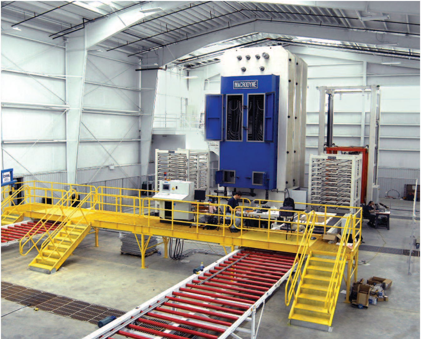
7500 ton, 10 daylight, heated platen press with vacuum enclosure and loading/unloading systems
