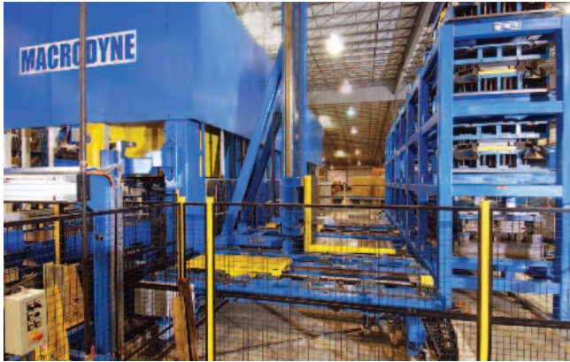
Hydraulic press line complete with Macrodyne automated die storage & retrieval system for twenty (20) 30,000 lb dies
