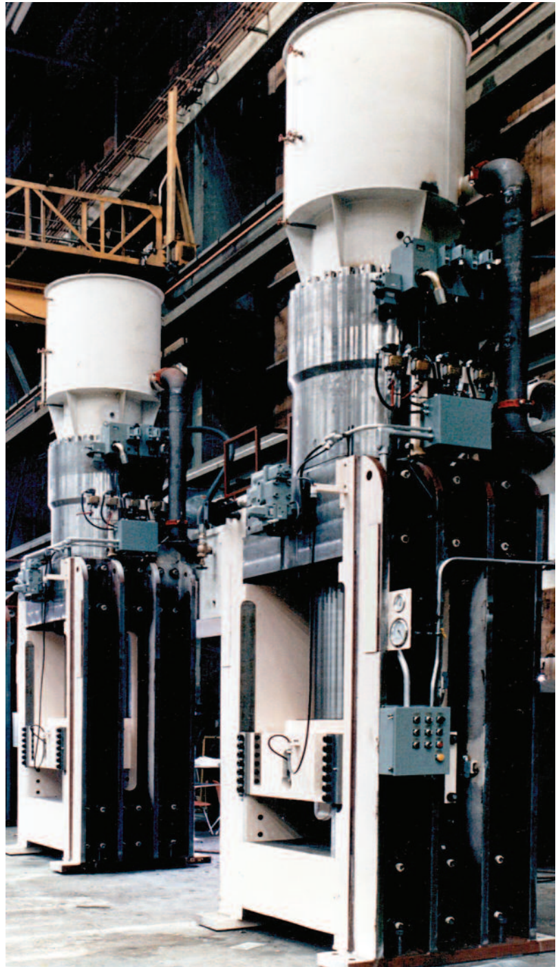
Two (2) 1000 metric ton pulp baling presses
