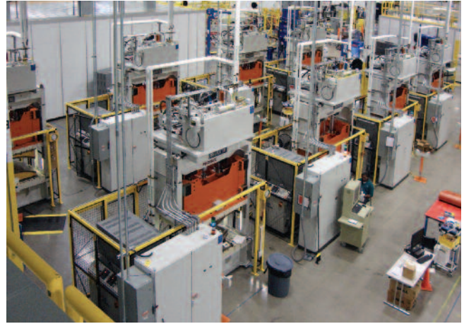
Sixteen (16) 100 ton advanced composite molding press lines
