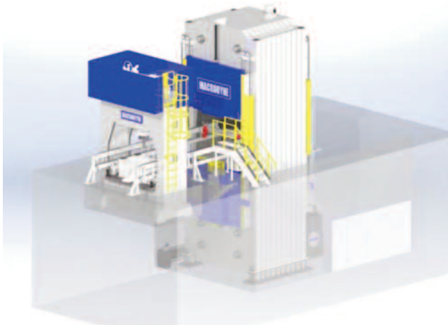
20,000 ton high pressure framing press system
