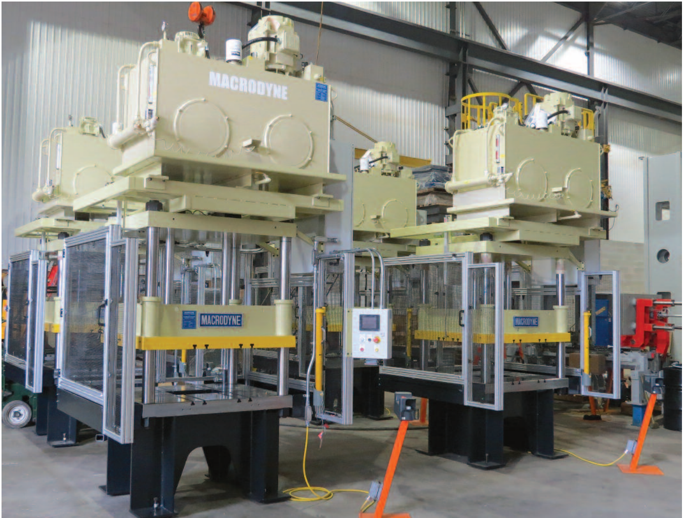
Four (4) 50 ton trim presses
