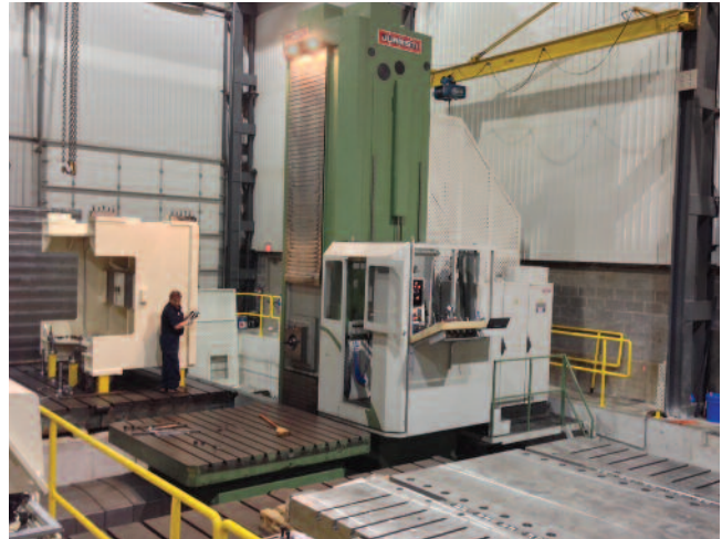
Large ram type boring mill
