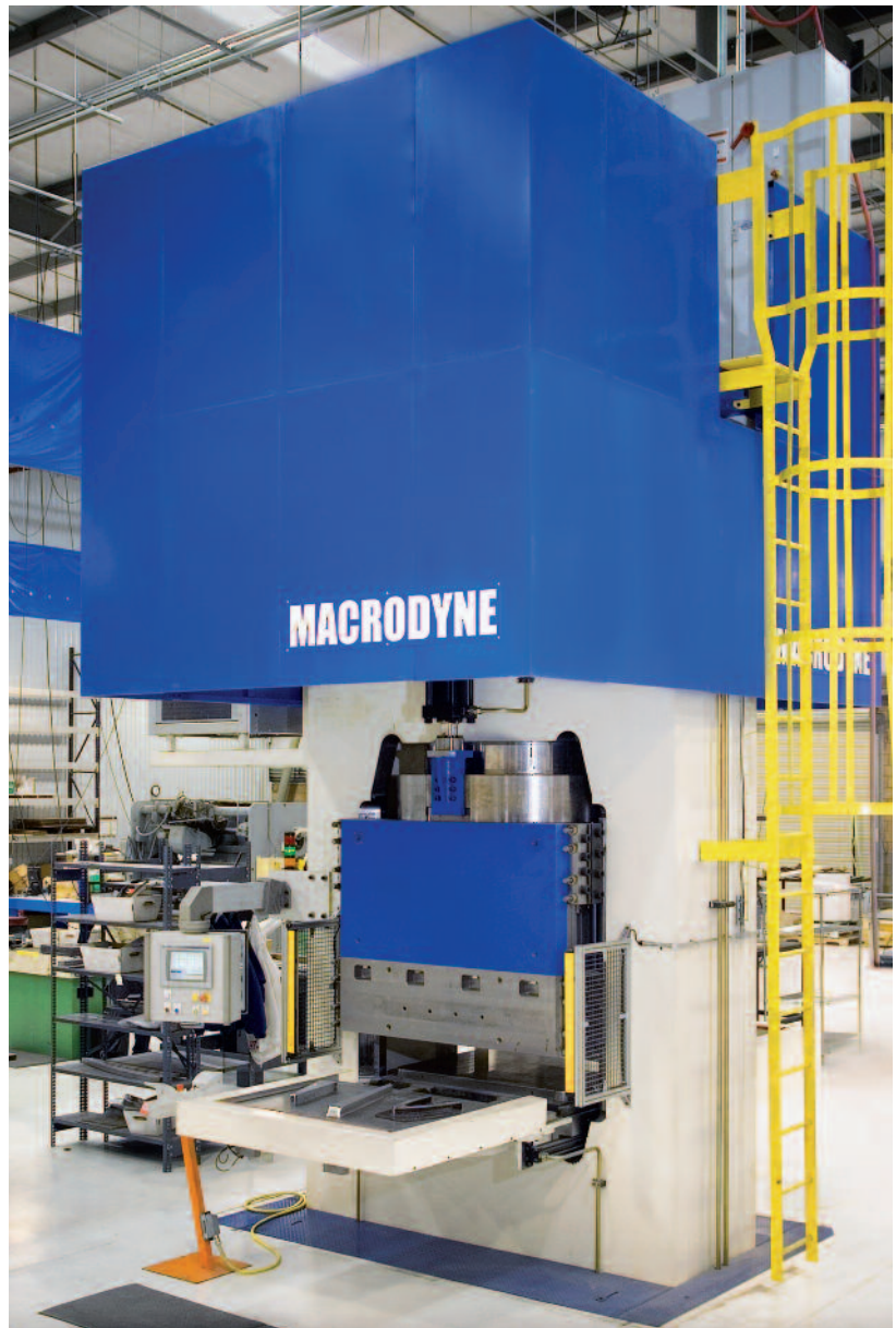
4000 ton elastoforming press with shuttle table
