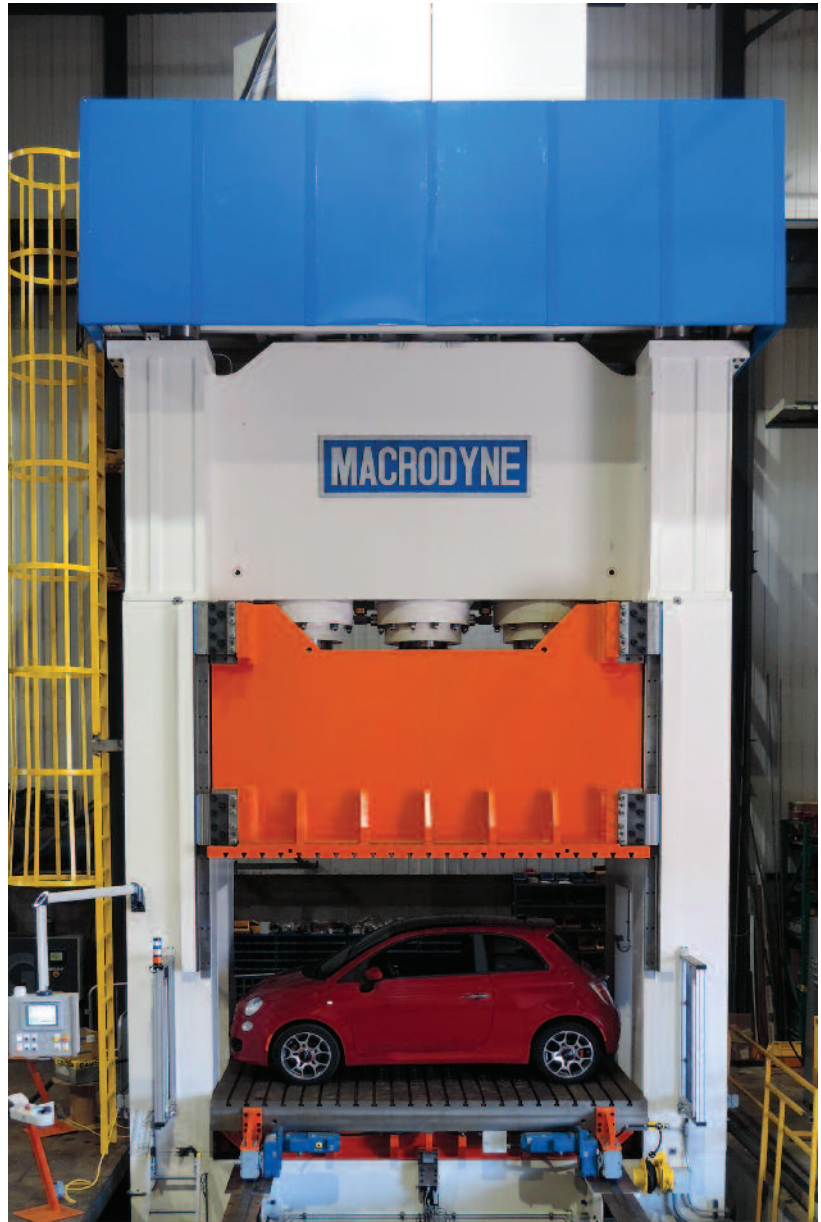
2000/400 ton single-acting pre-stressed housing style draw press with hydraulic cushion and rolling bolster
