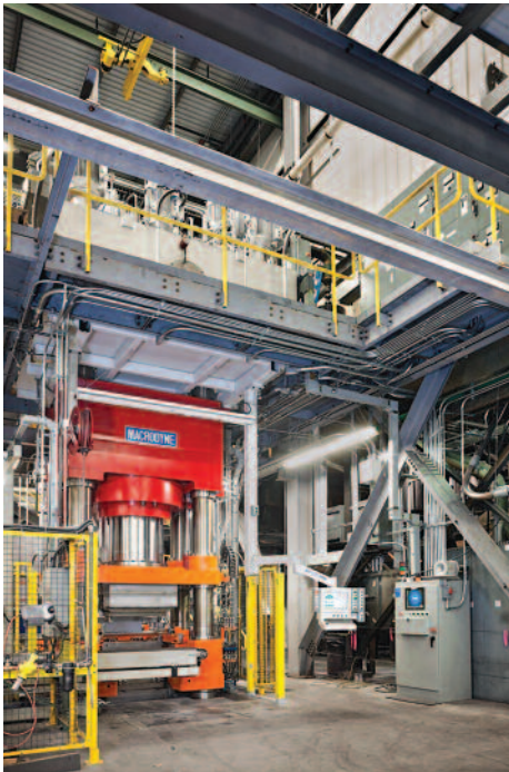
2250/130 ton compaction press for refractory brick
