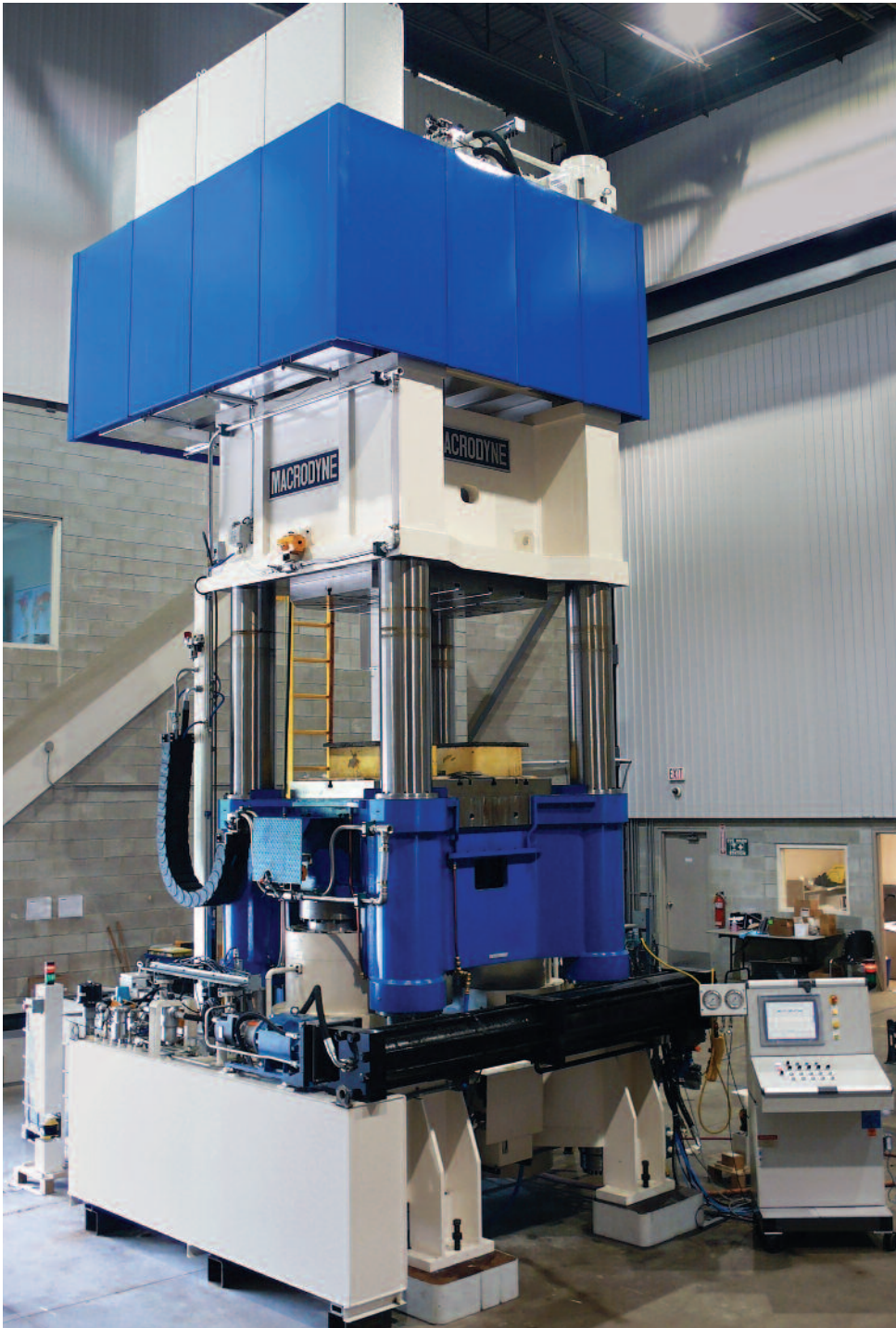
1400/225/50 ton triple-acting metalforming press with hydroforming package, high speed data acquisition system, and closed loop motion control
