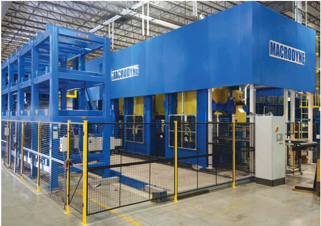
Macrodyne tandem press line for air conditioner panels comprising of one (1) 550/150 ton draw press, one (1) 200 ton press, two (2) 150 ton presses, destacker, five (5) feeders, exit conveyor, and fully integrated Macrodyne die storage & retrieval system
