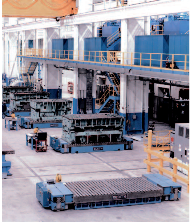
View of "T" type rolling bolsters in pre-staging area
