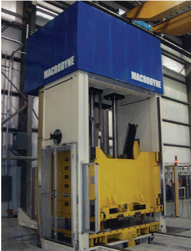
220 ton die spotting press with rolling bolster and 180 degree rotating platen
