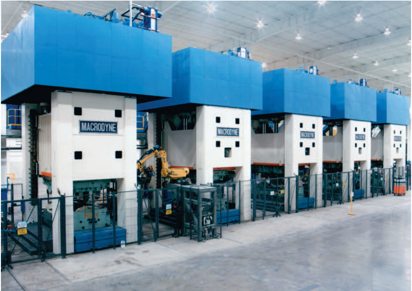
Press line for automotive body panels comprising of one (1) 2500 ton double-acting draw press with 500 ton NC cushion, four (4) 1250 ton single-acting presses, and six (6) robots for press loading, unloading and press-to-press transfer. Each press is equipped with two (2) 180" x 96" rolling bolsters in a "T" type configuration
