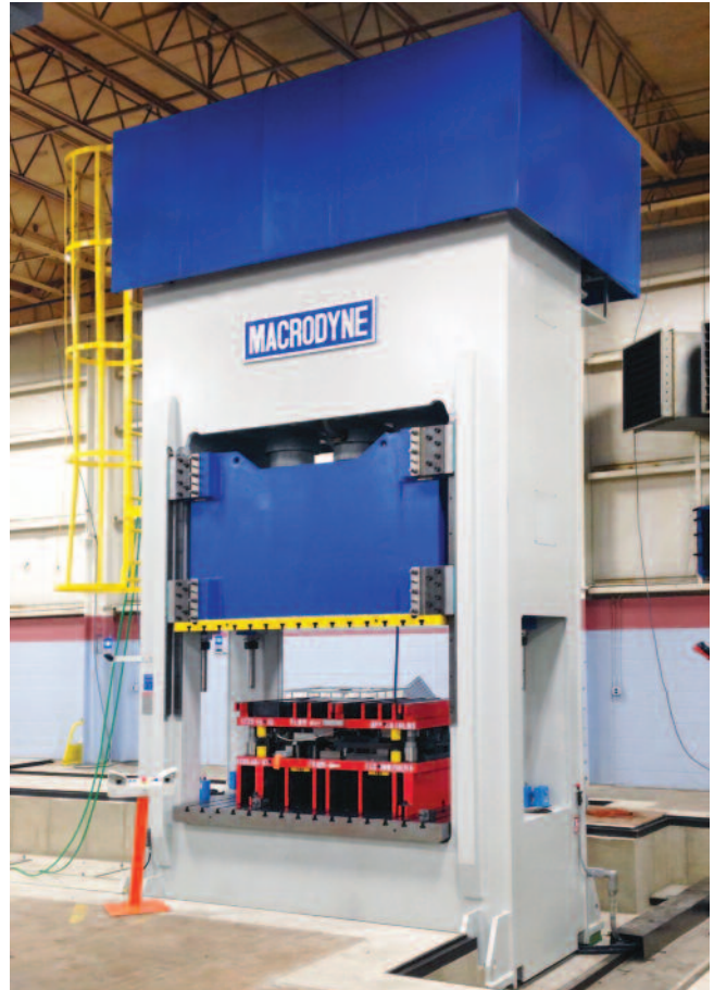
500 ton metalforming press with monolithic frame design
