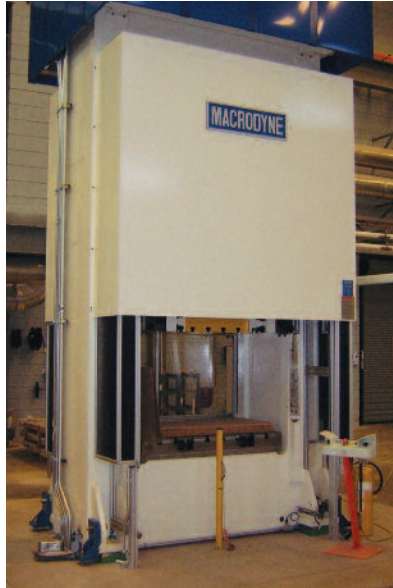
1200 ton squeeze casting R&D press
