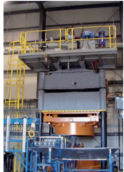
Rebuilt 750 ton cryofracture press
