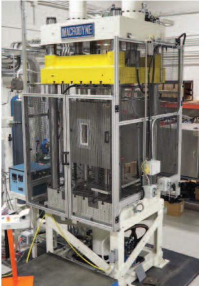
150/150 ton hot metal gas forming R&D press
