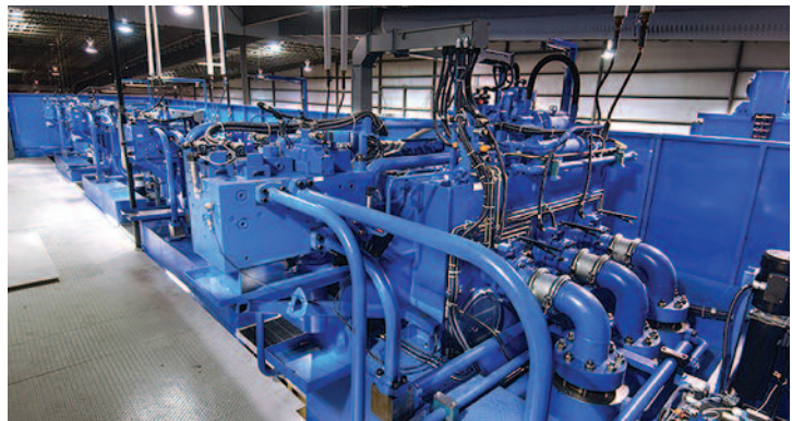
Hydraulic units for a Macrodyne tandem press line on a common platform
