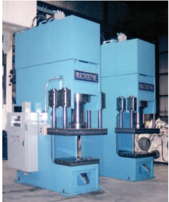
Two (2) 200 ton gap frame presses
