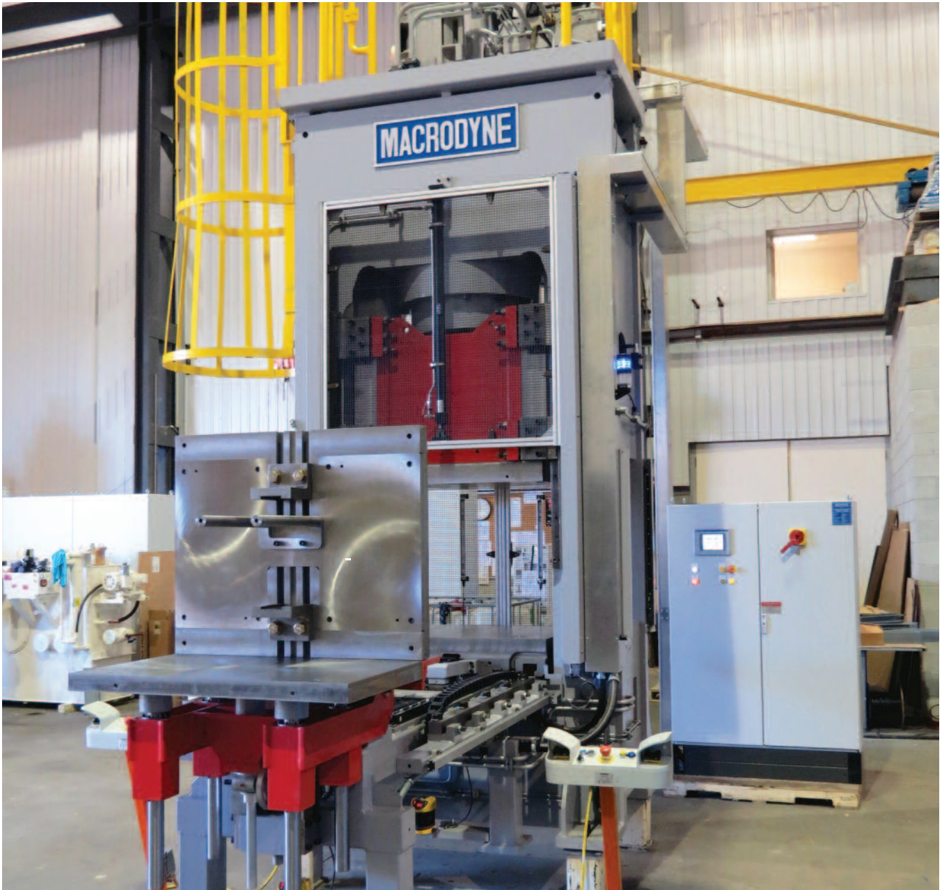
500 ton coining press with sliding/tilting table
