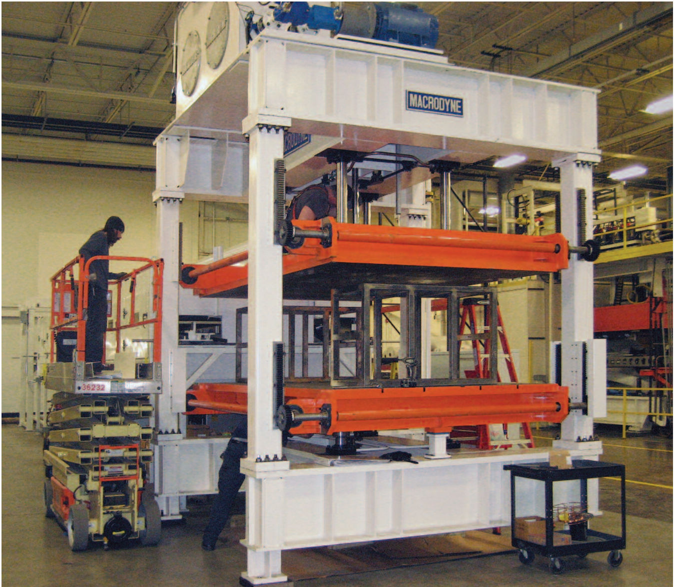
100/100 ton double-acting molding press
