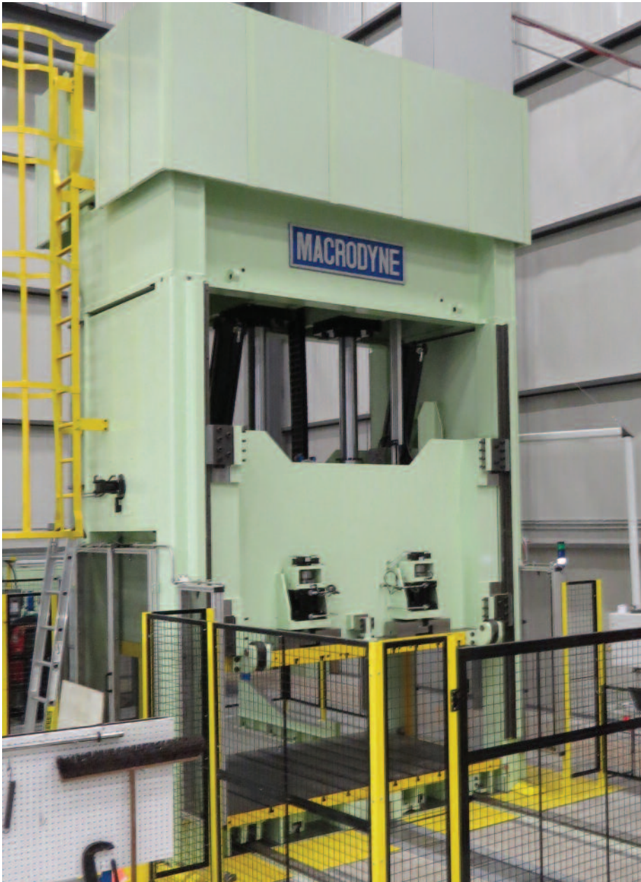
220 ton die spotting press with rolling bolster and 180 degree rotating upper platen
