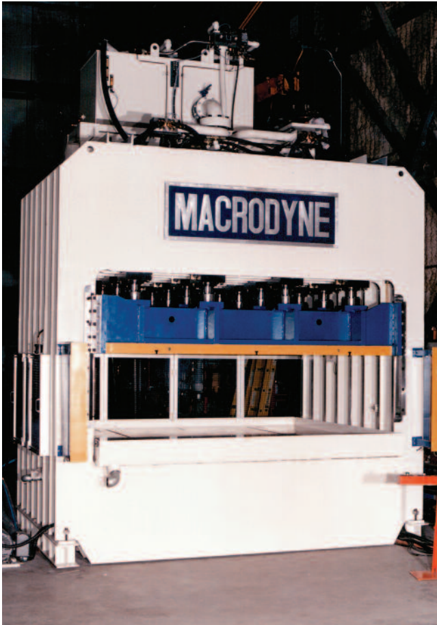
1500 ton hydroforming press with multi-frame design
