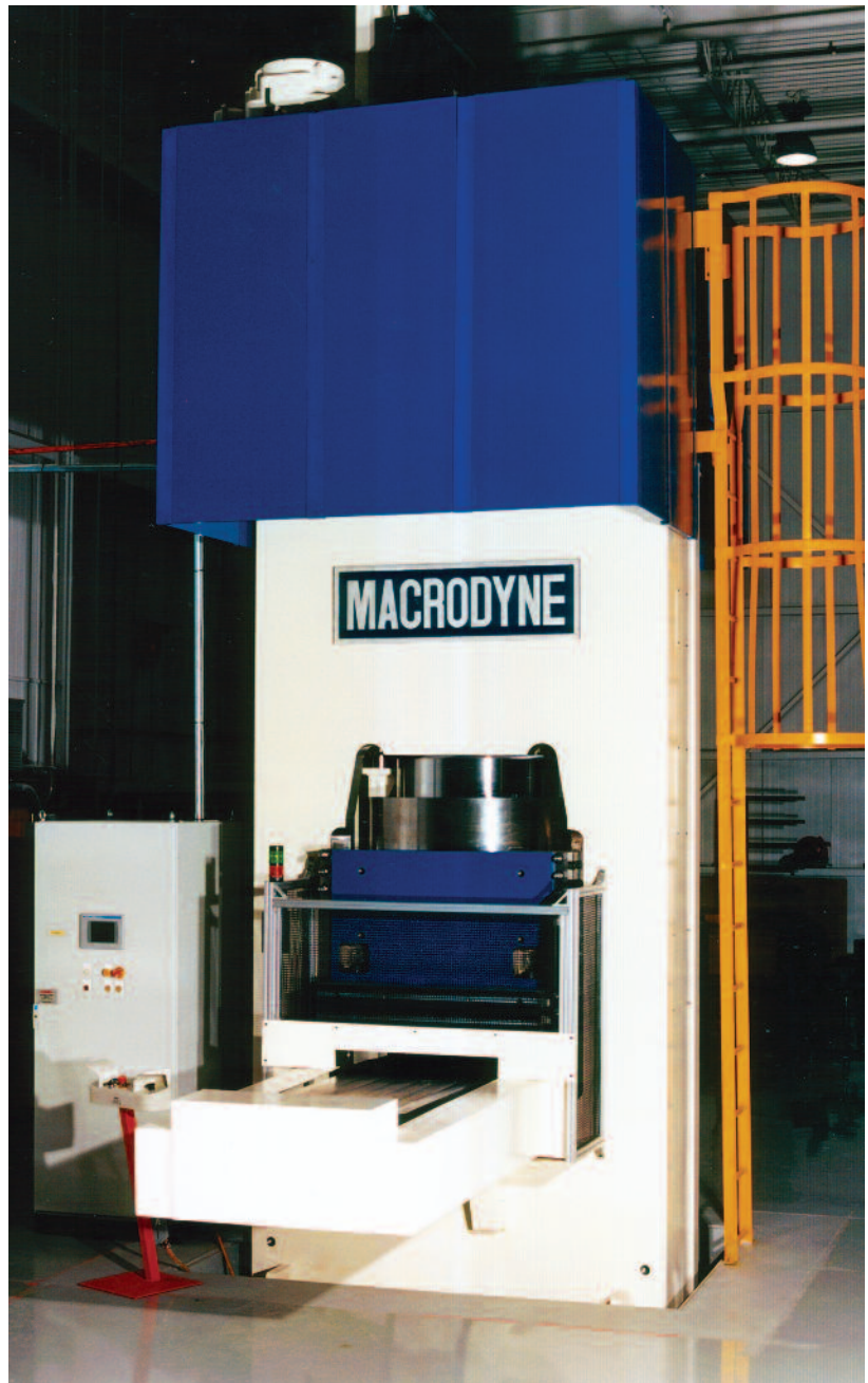
2000 ton elastoforming press with shuttle table
