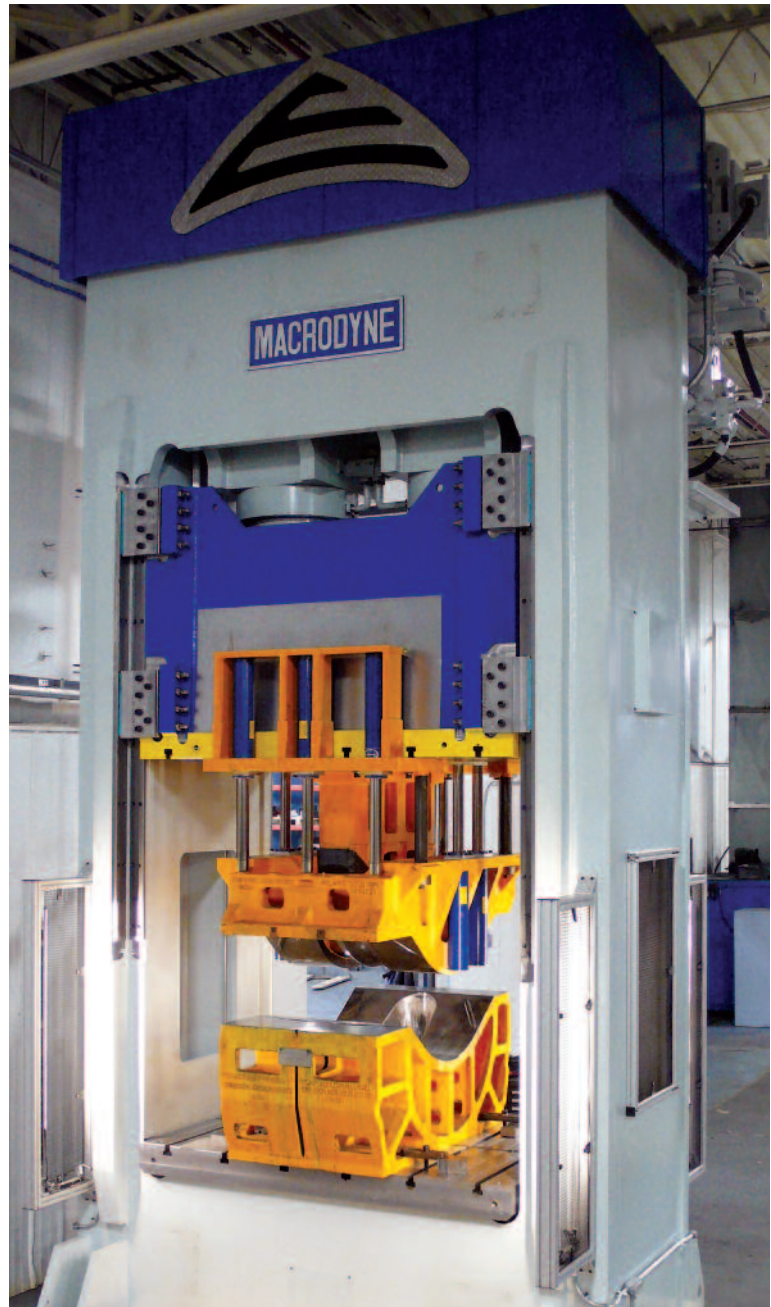
1500 ton metalforming press for the production of motorcycle parts
