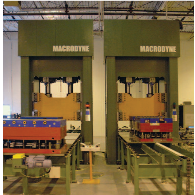
Two (2) 400 ton door embossing presses with quick die change systems
