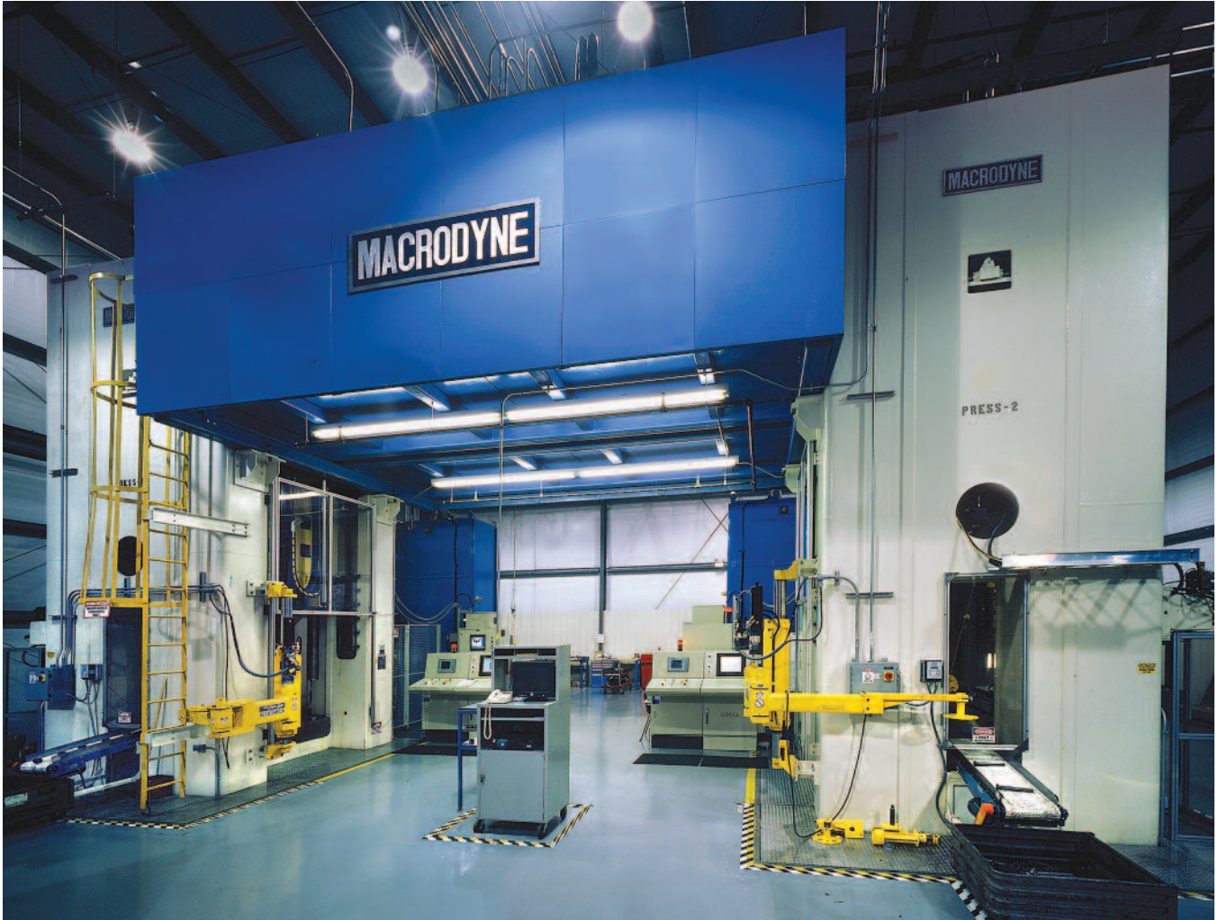
Two (2) 900 ton cold forming press lines, each comprising a 900 ton press, six (6) strippers and ejectors, 3-station transfer system, part loading robot, and hydraulic tool change arm
