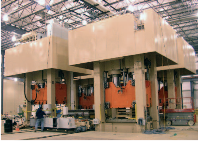
Four (4) 2500 ton SMC compression molding presses
