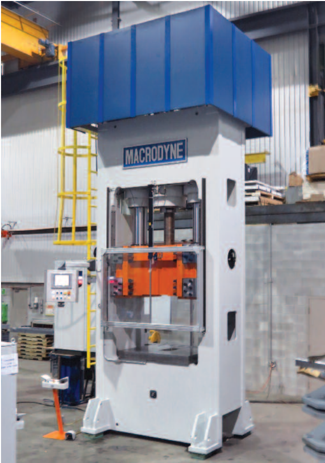
400/400 ton closed die forging press
